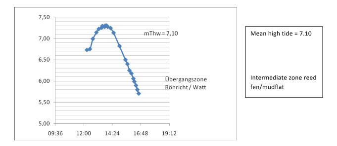
Fig. 7: Tidal curve for the Rodenkirchen level on 30.06.11<sup>38</sup>
