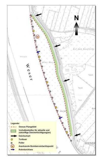
The limits of the planning area are defined by the land required for the expected dike repair as well as the mean low tide (MTnw). This means that the area's border to the east runs parallel to the present foot of the Weser dike at a distance of 25 m from this. In the west the border runs along the MTnw line (-1.57 m MSL).
